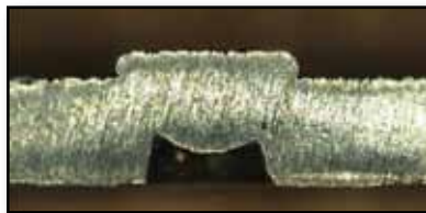
Figure 3. Projection Weld Cross-section (35X magnification)
